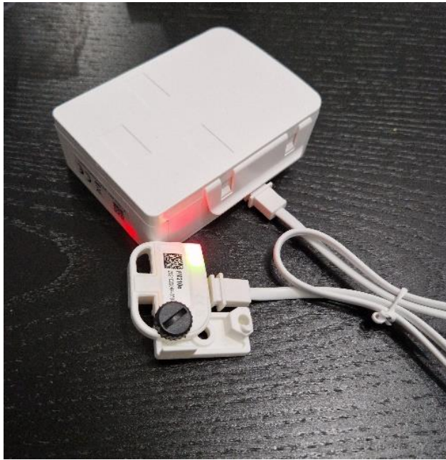
Figure 7 The Fludia energy meter tested in our office ©Hellenic Passive House Institute
