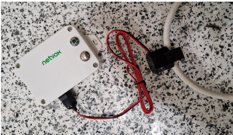
Figure 6 The netvox energy meter being tested in our office ©Hellenic Passive House Institute
