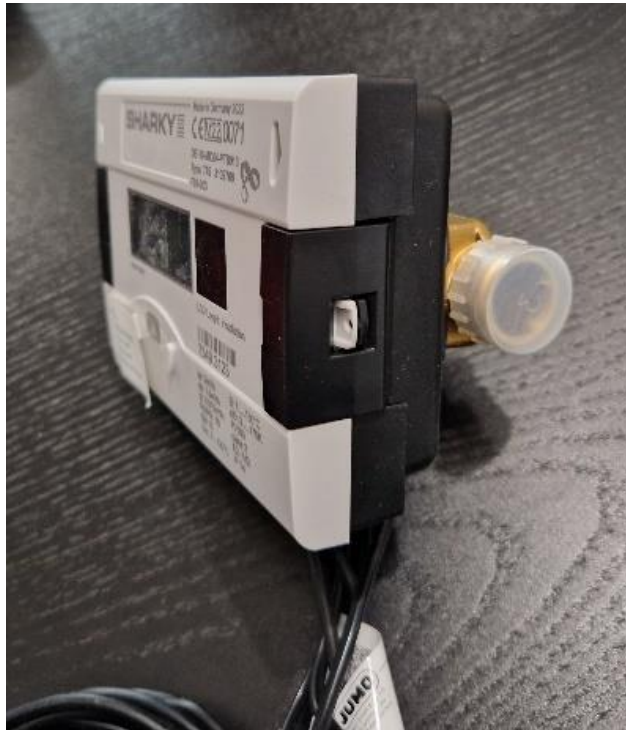
Figure 9 The Sharky 775 ultrasonic energy meter ©Hellenic Passive House Institute
