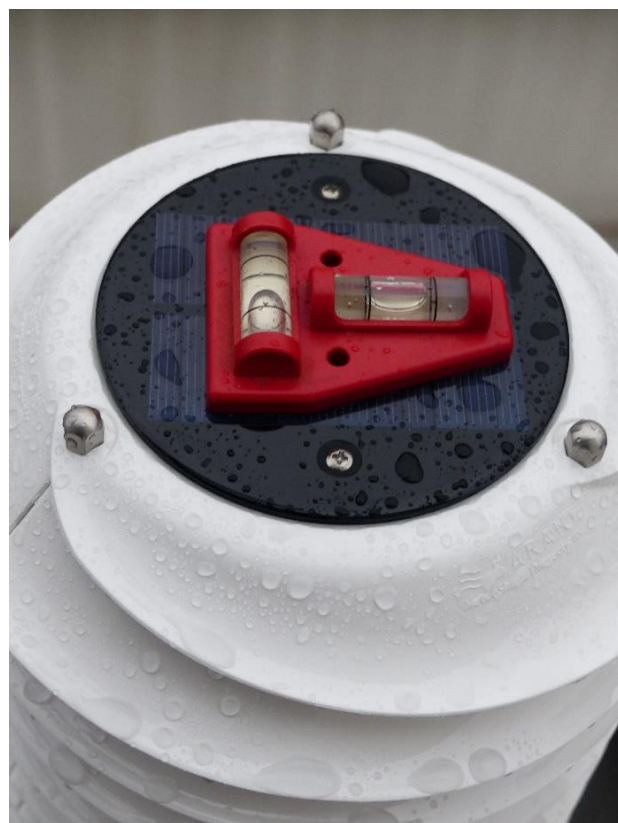
Figure 3 The weather station during installation with spirit level ©Barani Design
