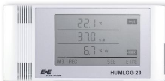
Figure 1: Data logger: Humlog 20 TCO (company E+E Elektronik)
