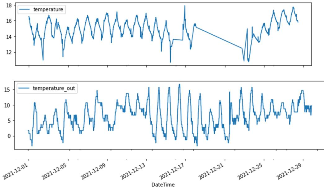
Even with outside temperatures close to 15 degrees in the warmer hours of the day, inside air temperature is always below 18 degrees.
