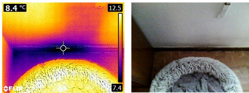
Connexion between wall and ground floor (north façade) @ VAND arquitectura
